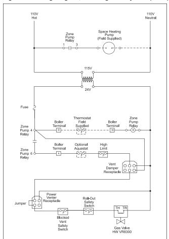
Figure 9d. Schematic, Standing Pilot System (BJVT).
